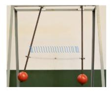
**4b)** Two pendulums are connected by a light spring. What happens if you pull one of the pendulums to the side and let it go?
