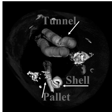
(alder) showing the shipworm wood. Note the shell (arrows), pallets.
